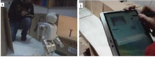
Fig. 9. Demonstration of the proposed teleoperated system on a 'lunar scenario' a) Robot HOAP-3 and a human operator work collaboratively on finding and moving the 'antenna'. b) The operator teleoperates the robot with the HMI using a pocket PC.
