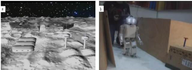
Fig. 2. a) the recreation of lunar scenario. b) HOAP-3 teleoperated through a corridor looking for the 'antenna'.
