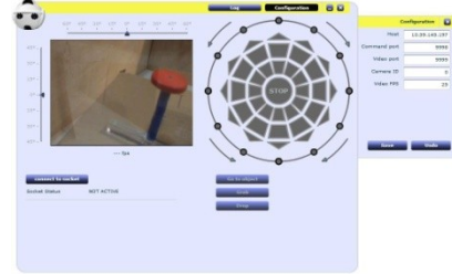
Fig. 1. The HMI for teleoperation of robot HOAP: On the left there is the video panel and the head movements controls. On the right side of the HMI there is the communication configuration panel. On the bottom side there is the ‘connect’ button and the communication log. On the center wheel of the HMI there are the walking and turning movements’ controls and the higher order command buttons, ‘Go to object’, ‘Grab’ and ‘Drop’.
