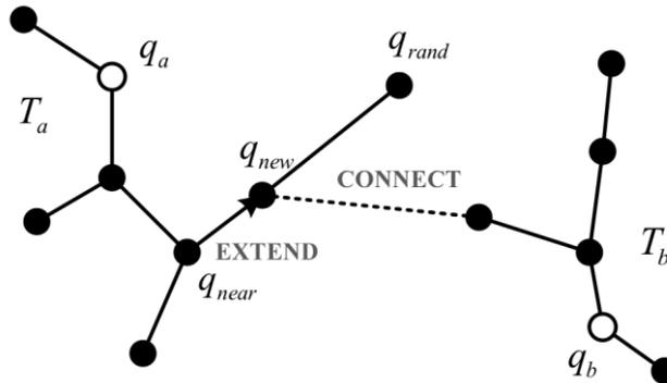
Fig.3. Process of RRT-Connect merging two RRT trees
