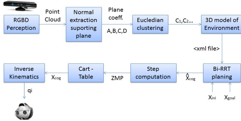
Fig.4. Schema of the proposed architecture. The output of each step is represented within the arrows.
