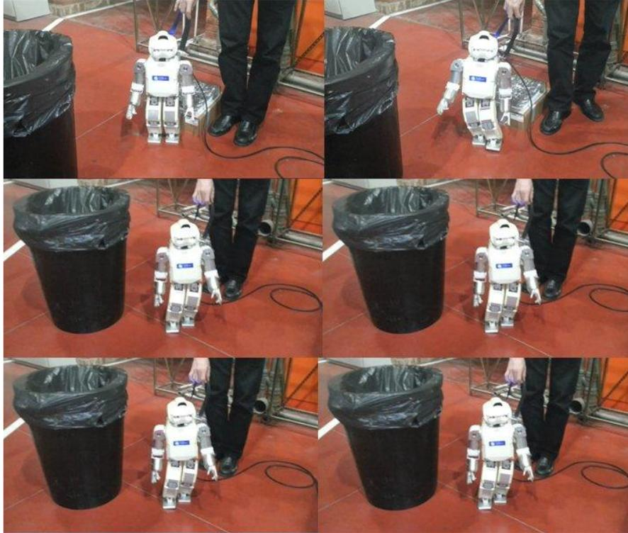
Fig. 8. Several frames representing the real performance of the robot path planning in the laboratory. The black bucket is one of the obstacles avoided.
