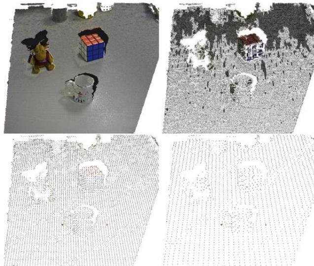
Fig.1. Down-sampling the point cloud using voxelgrids at different sizes. Leaf sizes are 0.005m, 0.01m, 0.05m and 0.08m respectively
