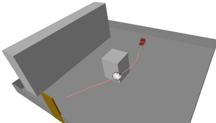
Fig.7. Path planning COG result plotted in OpenRave. HOAP head represents the COG of the complete robot.
