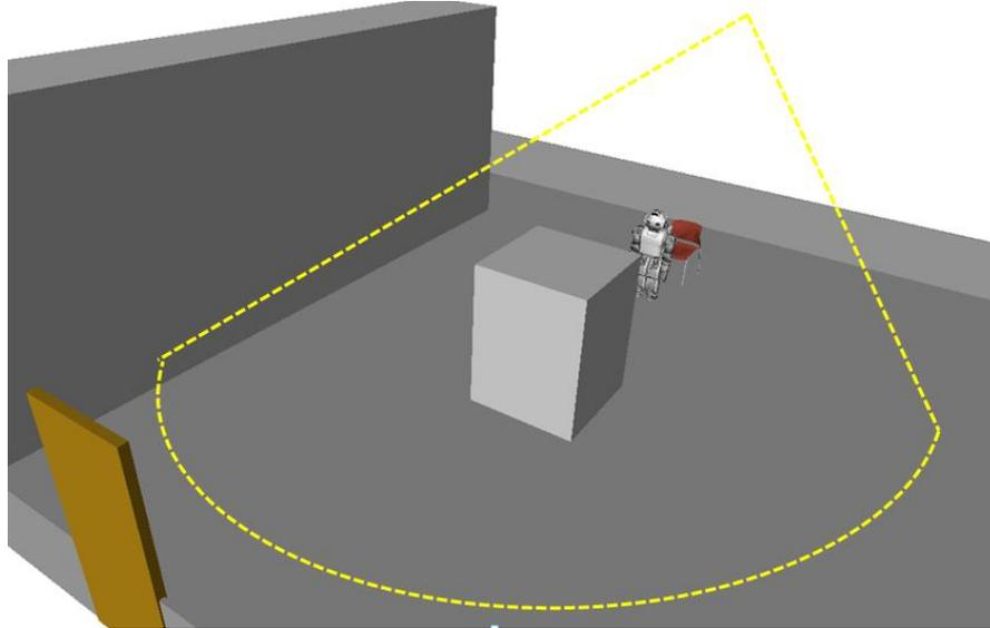
Fig.6. Simulation of the environment with bounding boxes representing obstacles detected by the RGB-D sensor. Yellow dotted line represents the field of view of the RGB-D sensor.
