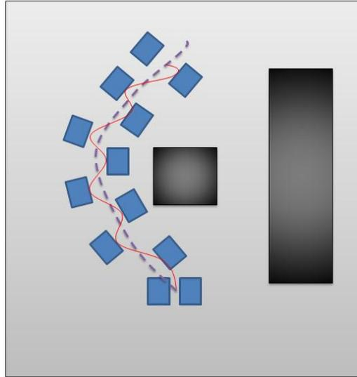
Fig.5. Top-view schema of the complete scenario with obstacles in dark gray, global path planning represented by the dotted line, steps plotted as blue boxes and finally COG path shown with a red thin line.
