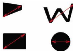
Fig. 2. How to measure robot foot dimensions
